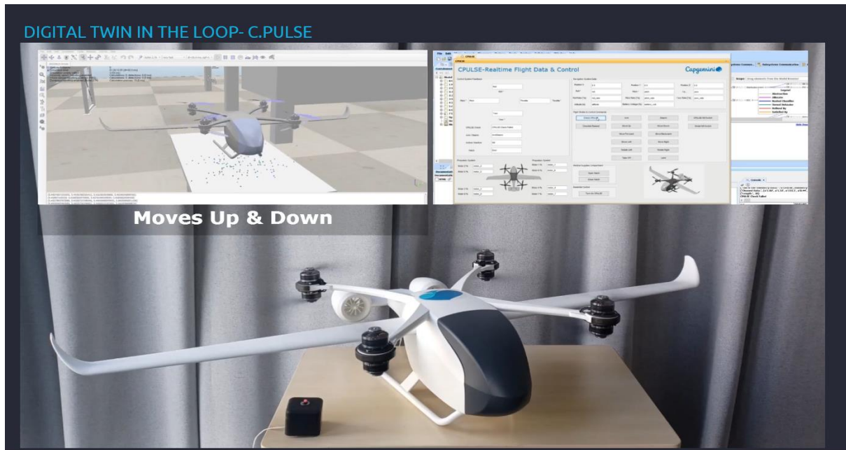
Figure 26 - Cameo Simulation Integration with Prototype HW
